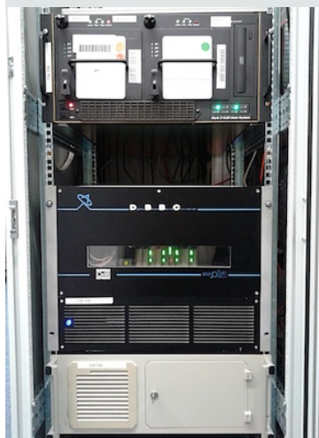
DBBC: From top to bottom the Mark5B+ data recorder, the DBBC, and the control PC.
